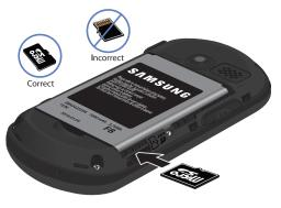
Replace the cover by lining up the tabs and then firmly pressing the cover down until it snaps into place. Check that the battery is still properly installed before turning on the phone.
